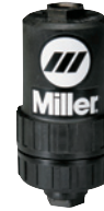
In-Line Air Filter Kit 228926 Mounts to the back of the AirForce® 27i and 40i. Includes male and female 1/4-inch NPT quick disconnect fittings and hose for easy on/off connection. The replaceable filter element filters to .85 microns.
