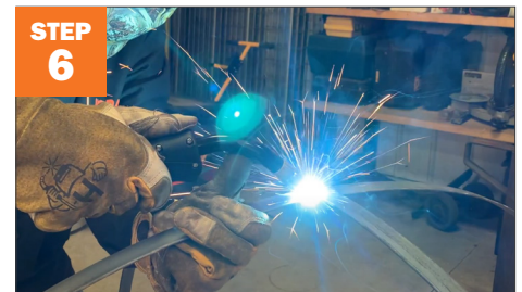
STEP 6 Weld second ring.
