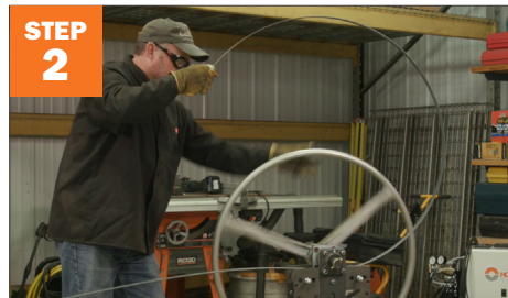
STEP 2 Form flat bar into a ring with a roller or by hand.
