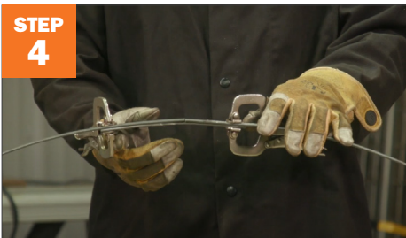
STEP 4 Use scrap flat stock & clamps to secure ring ends together.
