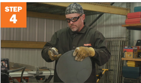
STEP 4 Clean up and smooth the edges of the metal. Tip: Use a hammer on the edges before using a flap wheel
