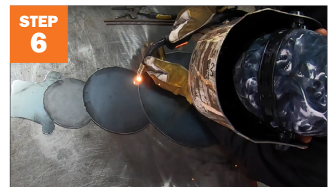
STEP 6 Lay out pieces facedown and tack weld.
