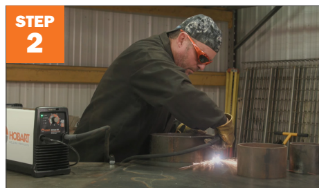
STEP 2 Plasma cut three circles for the snowman. Tip: Use a pipe as a guide
